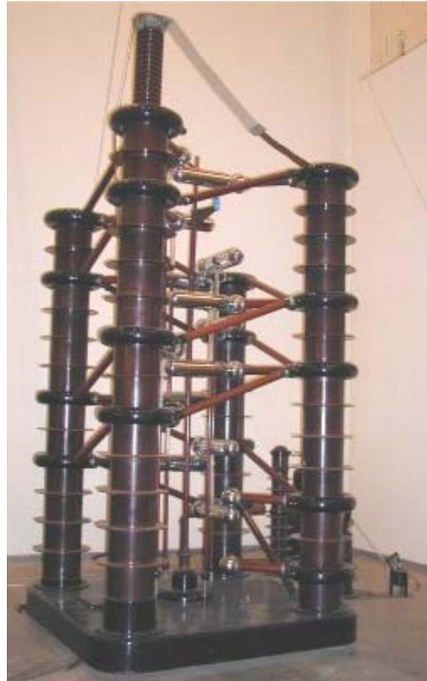
Fig. 4.10: 8- stage impulse generator
