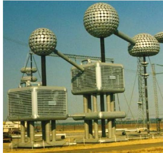
Fig. 4.3: Cascade connected test transformers
