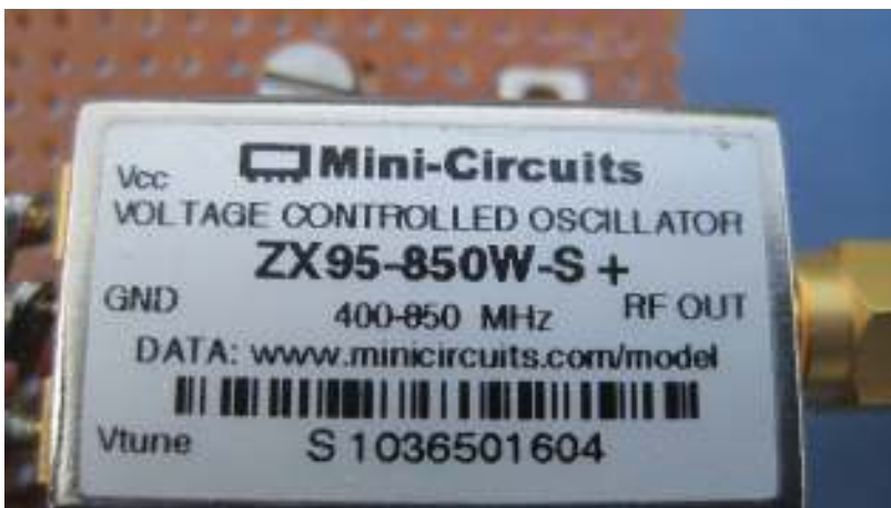
Figure 6 Voltage tuned oscillator, VTO, (Mini-Circuits) attached to the line
