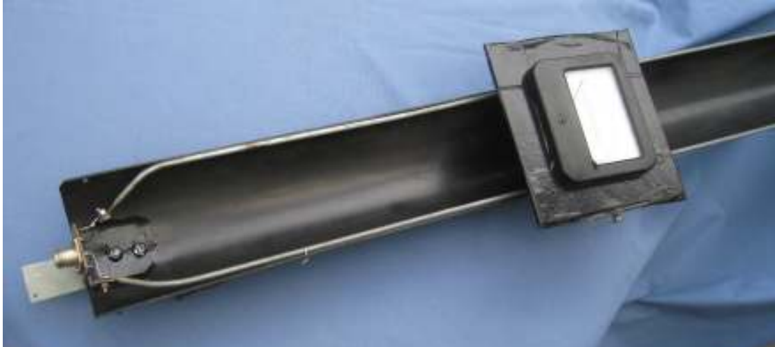
Figure 3 Lecher Line apparatus (rod diameter, d = 5.0 mm, separation 10.5 cm)
