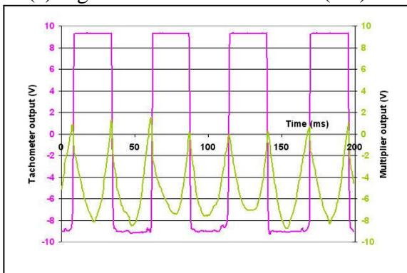
(b) signals from the tachometer (red) and the mixer (green)
