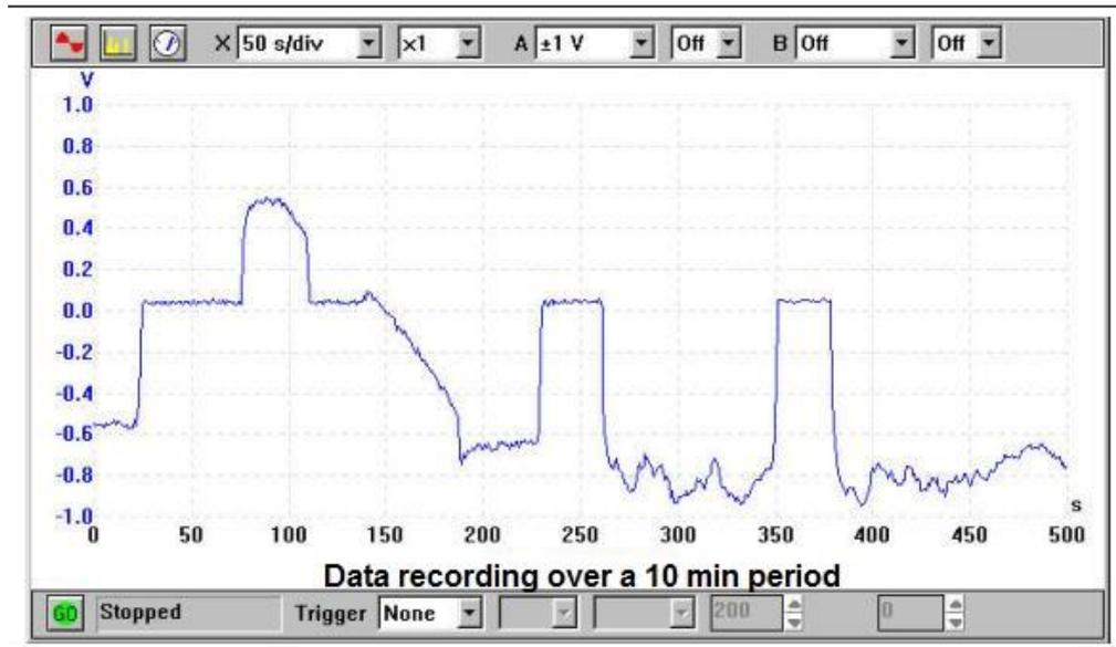
Figure 8 Earth's electric field changes as a thunder storm was approaching (rotor covered for periods 30 –70 s, 107-140 s, 230-260 s and 350-380s )
