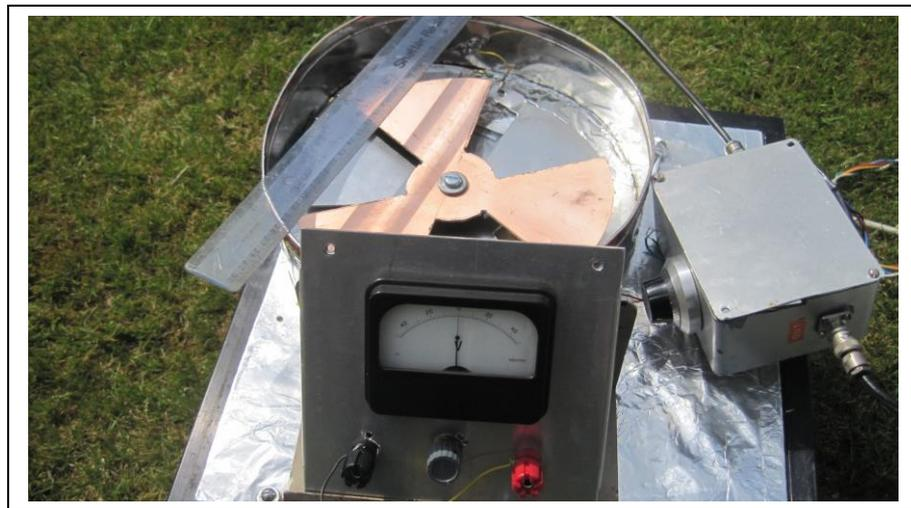
Fig 4 Fieldmill with separate charge amplifier and meter resting and on the case (ruler indicates the size of the apparatus)
