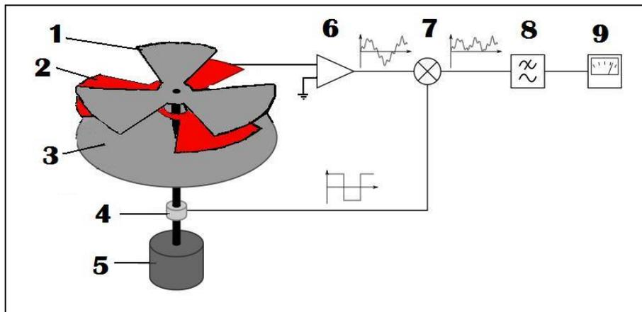
Figure 2 Diagram of a typical Fieldmill with electronic circuitry
