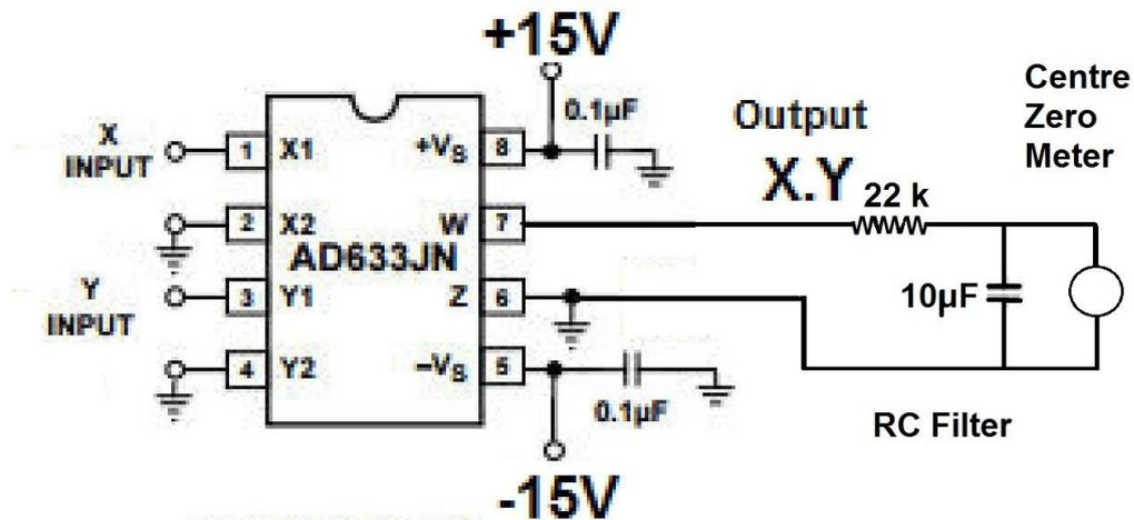
Figure 5 Multiplier circuit for **mixing** the tacho and charge signals ( X and Y ) (detailed circuits of the tachometer and charge amplifier are available on request)
