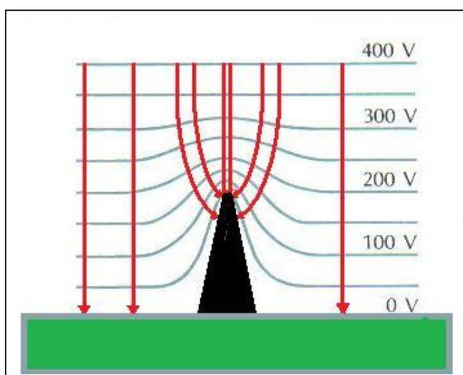
Figure 1 Distortion of field lines round a conducting object (blue – potential, red – field)
