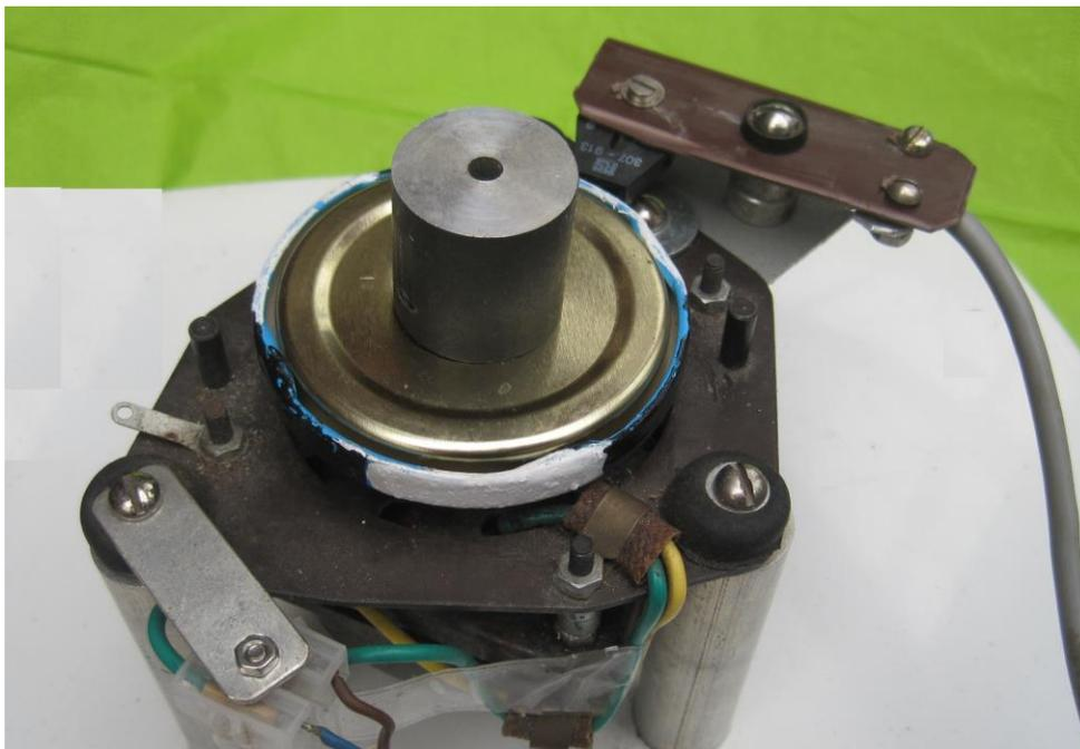
Fig 3 Photograph showing the motor plus tachometer
