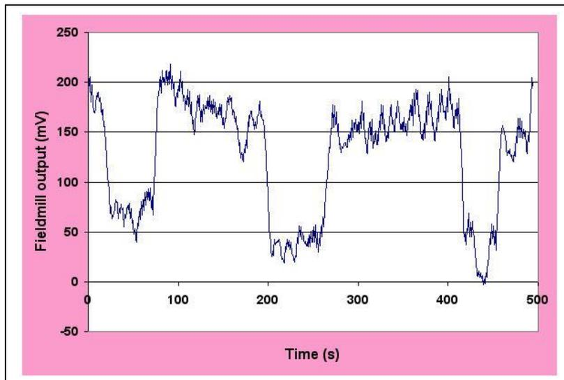
Figure 7 Output from the Fieldmill (rotor covered with earth plate during low readings of about 50 mV – this is an instrumental off-set error)
